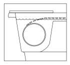
The underwater standard slat system can be installed in pools from our Monaco and Antibes ranges. The standard set includes a 140 Nm-24-IP68 fiberglass roller with pool-wall fixings, a motor control key box, a fixing kit for roller tube straps, and a 110 x 65 mm aluminium beam for top-down wood support. This cover system works with standard, 10-12 cm water-level systems.
